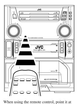
the remote sensor on the front panel.
